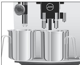
When the JURA is switched off, the system is automatically rinsed if a speciality coffee has been prepared. If milk has been prepared, you will also be prompted to clean the milk system.
